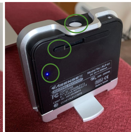
Left to right: blue light, aperture slide, aperture
